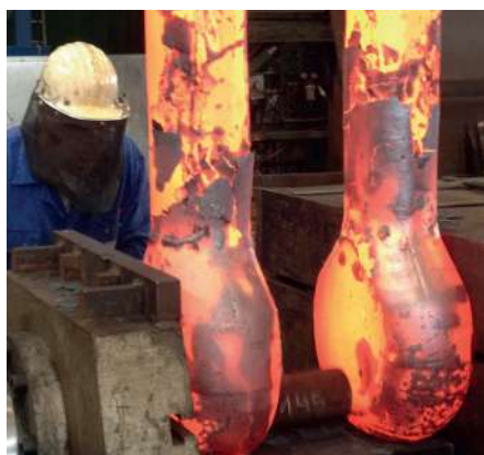
Bow forging dimensions are controlled and adjusted
