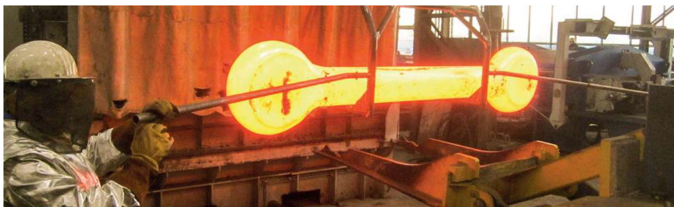
Zero-waste forging process: 'dog bones' are formed to bow shape
