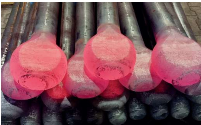
Zero-waste forging process: eyes are upset forged
