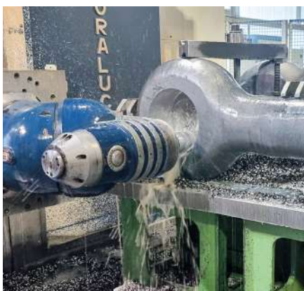
Shackles and pins CNC machined in-house
