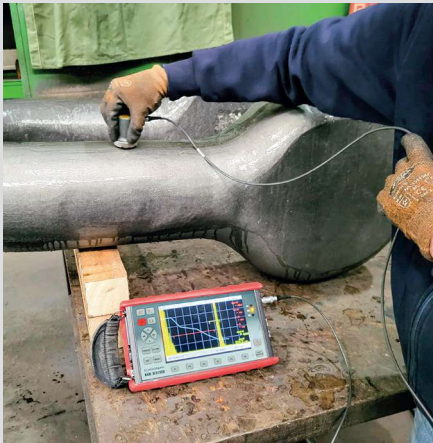
NDT - ultrasonic testing
