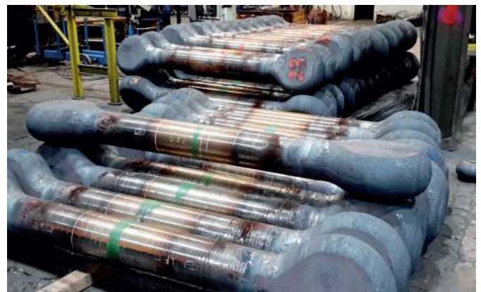
Zero-waste forging process: 'dog bones'
