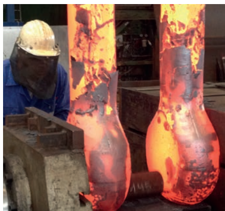
Bow forging dimensions are controlled and adjusted
