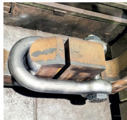
Shackles are proof load tested (witnessed by Classification society on request)
