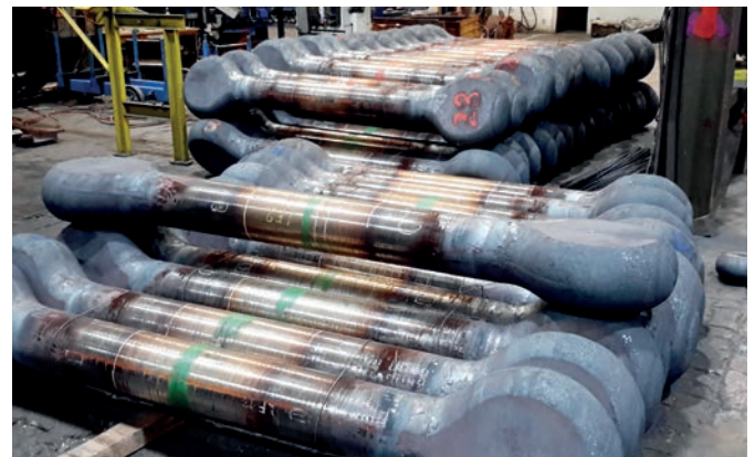
Zero-waste forging process: 'dog bones'
