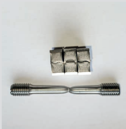
Mechanical testing is performed for every production batch and ensures individual traceability to every shackle.
