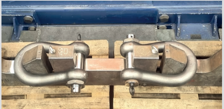
Proof testing (2 x WLL) on in-house 3000 t test rig using quick release system
