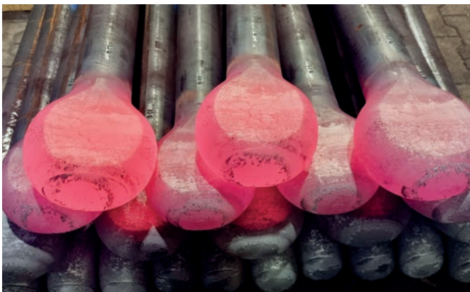
Zero-waste forging process: eyes are upset forged
