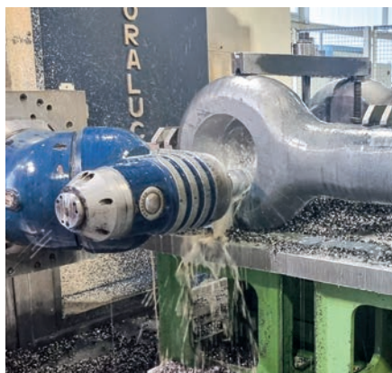
Shackles and pins CNC machined in-house
