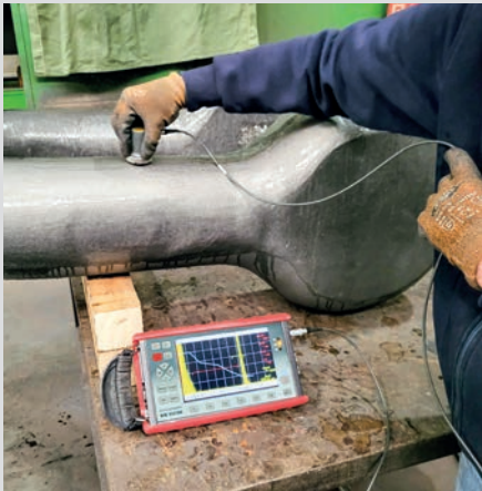
NDT - ultrasonic testing
