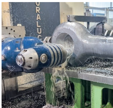
Shackles and pins CNC machined in-house
