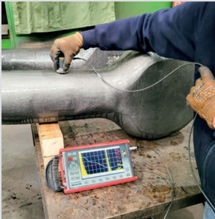
NDT - ultrasonic testing
