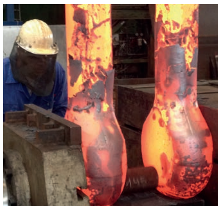
Bow forging dimensions are controlled and adjusted
