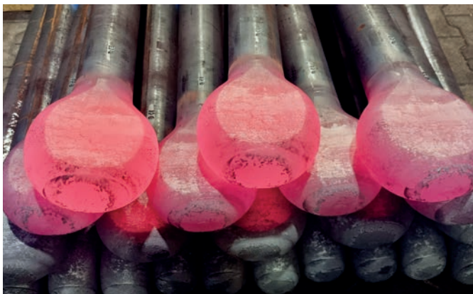
Zero-waste forging process: eyes are upset forged
