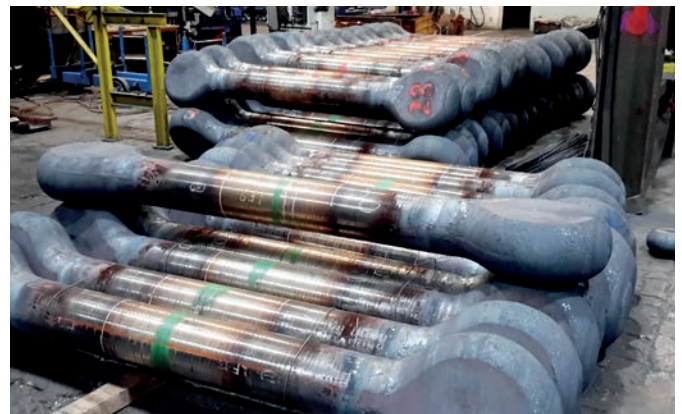
Zero-waste forging process: 'dog bones'
